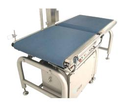
The extra wide 628mm belts are driven by stainless steel drum motors ensuring strong, reliable and consistent power to transfer heavier trays, boxes and cases. The surface finish of the belts is sufficiently durable and provides a positive grip for regular weights of up to 60kg.
